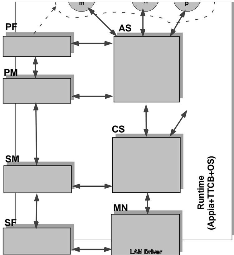
Figure 1.1: Architecture of a MAFTIA Host
